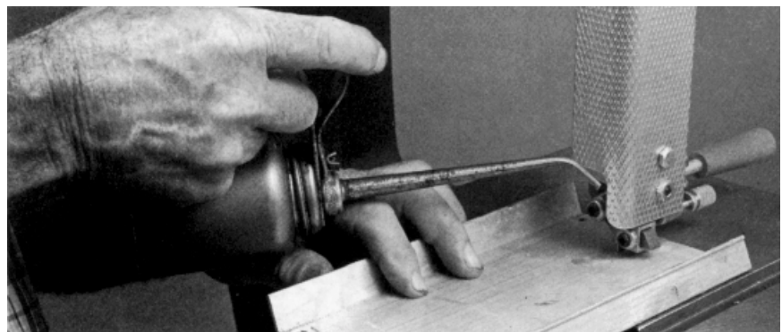
Figure 14-45. When cutting metal, apply oil to the cutting line to help keep the blade from overheating.
